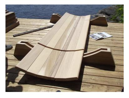
Fill the cradles with enough staves to hold the middle section with the door, and the corresponding back middle section.
