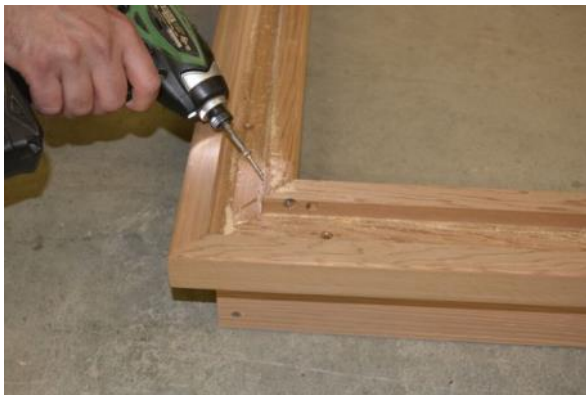
Angle-screw corners to draw tight
