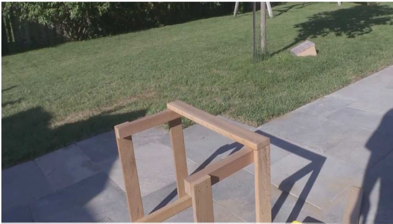
67. Assemble the two sides and front of heater guard using 1 1/2" screws.
