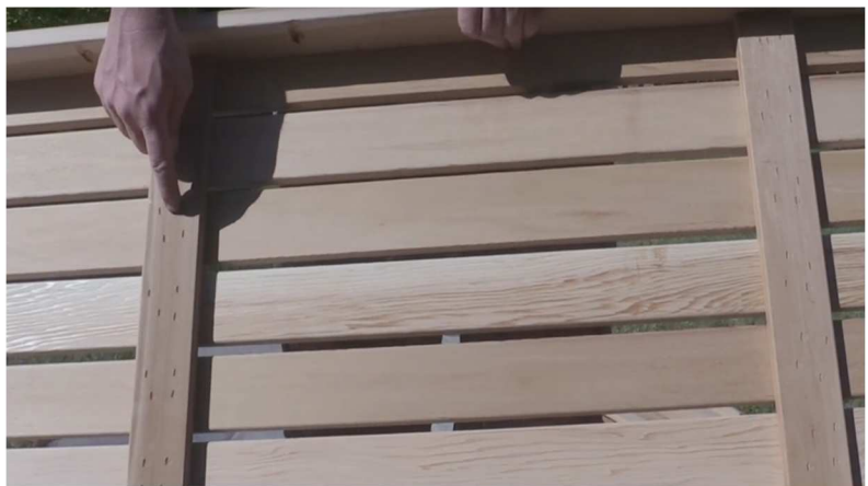
54. Make sure to line up the bench crossbars with the seat supports.
