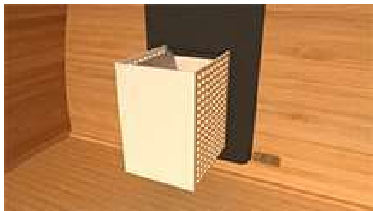
Inlet beside wood heater on Back wall
